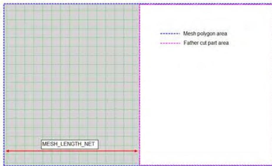
Tekla Structures size inquiry gives the size so that it gives the height first and the width last, whereas MESH\_SIZE\_NET reports the width first and the height last: 20/8-100/200-**5950/2950**.
