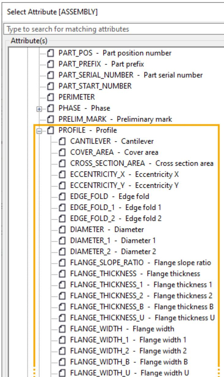
For example, MAINPART.PROFILE.HEIGHT with the ASSEMBLY content type shows the height of the main part profile in the assembly.
