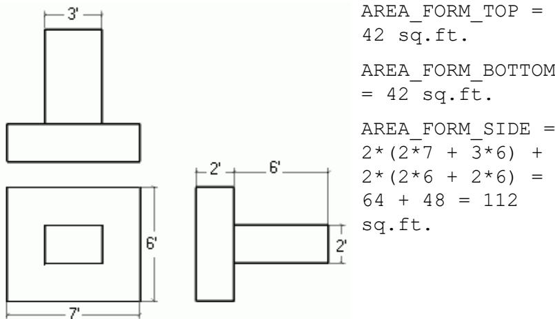
To report the formwork areas of cast-in-place cast units, use the [template attributes \(page 19\)](#) `AREA_FORM_TOP_GLOBAL`, `AREA_FORM_BOTTOM_GLOBAL`, and `AREA_FORM_SIDE_GLOBAL` with the `CAST_UNIT` content type. With these `..._GLOBAL` attributes, **Top-in-form face** settings have no effect.
