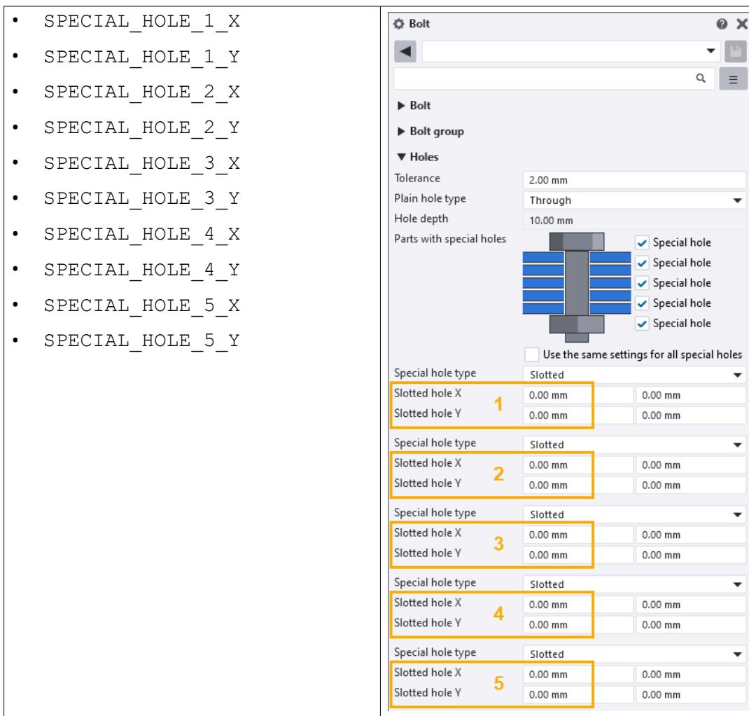
The x and y allowances comply with the x and y directions of the bolt group.
